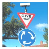
In addition, each approach to the mini-roundabout would require 'Give Way' road markings in conjunction with the appropriate illuminated 'roundabout ahead' and 'Give Way' signs shown opposite.. The amount of verge lost to provide the road space required for a mini-roundabout, by comparison to a 'give way' junction arrangement, is also likely to be an issue.
